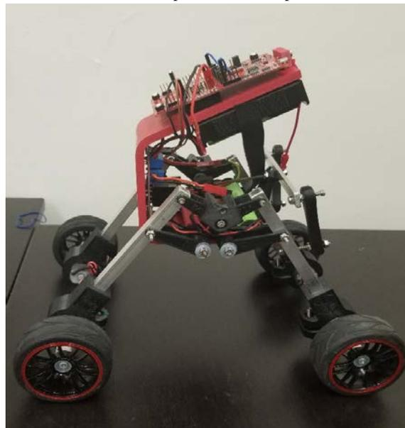
Fig. 7 Fully Assembled DSTR Robot
