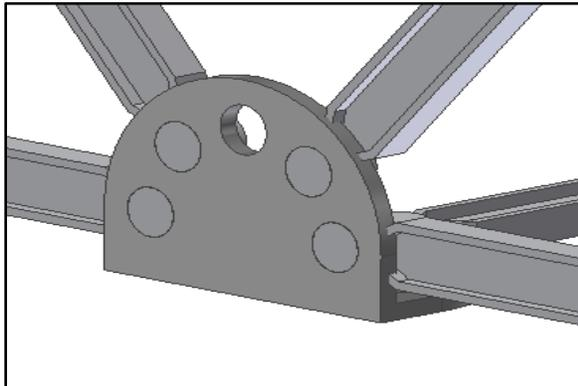
Fig. 5 Gusset Plate in Simulation
