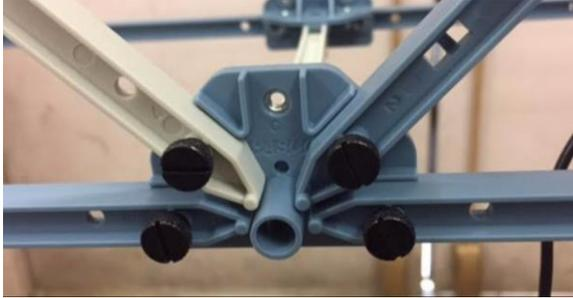
Fig. 3 Gusset Plate in the Experiment
