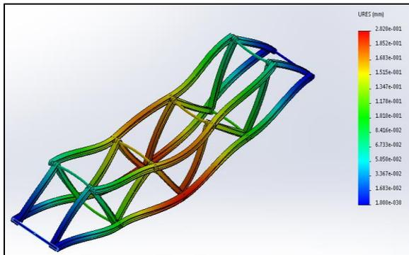
Fig. 6 Displacement of Pin-Jointed Truss
