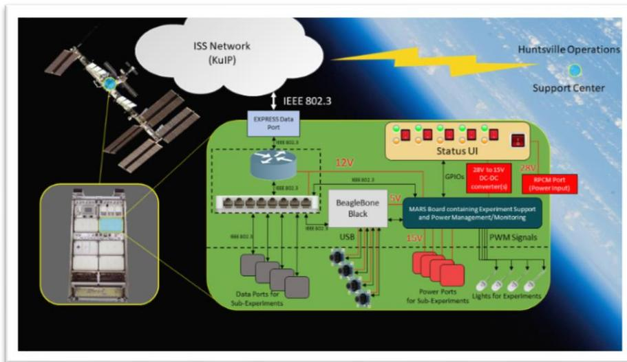
Fig. 1 Conceptual Block Diagram for the Hermes Facility
