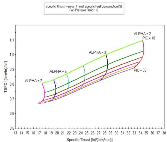
Figure 4 Carpet Plot of TSFC vs Specific Thrust
